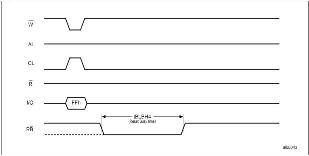
Figure 25. Program/Erase Enable waveform
