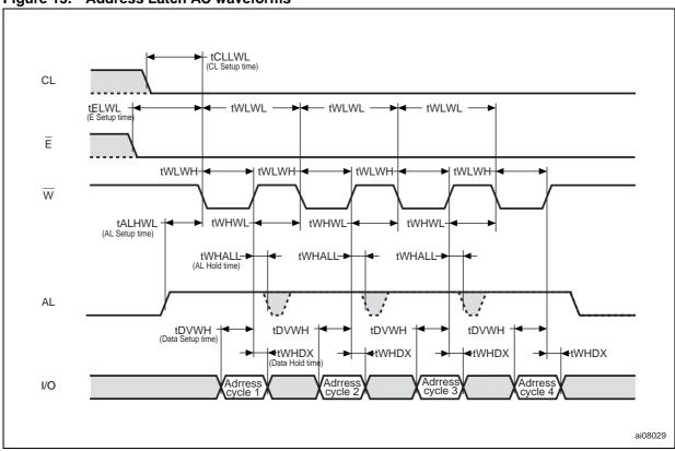
Figure 16. Data Input Latch AC waveforms
