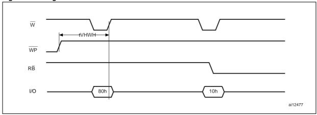
Figure 26. Program/Erase Disable waveform
