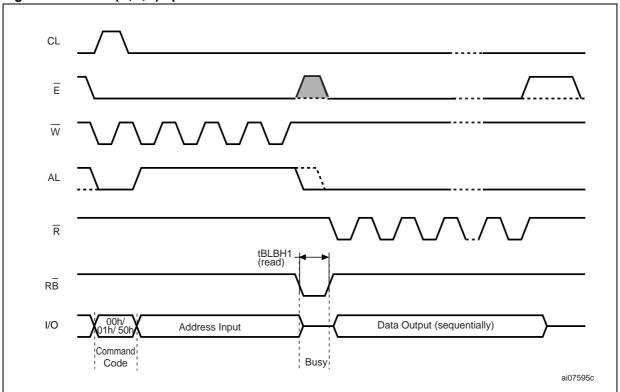
Figure 6. Read block diagrams
