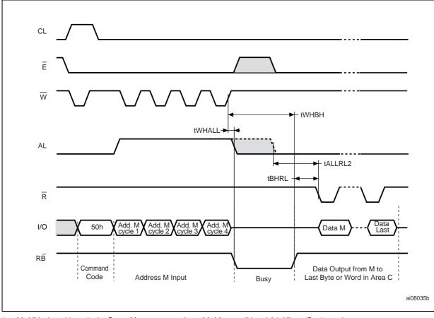
Figure 21. Read C Operation, One Page AC waveform
